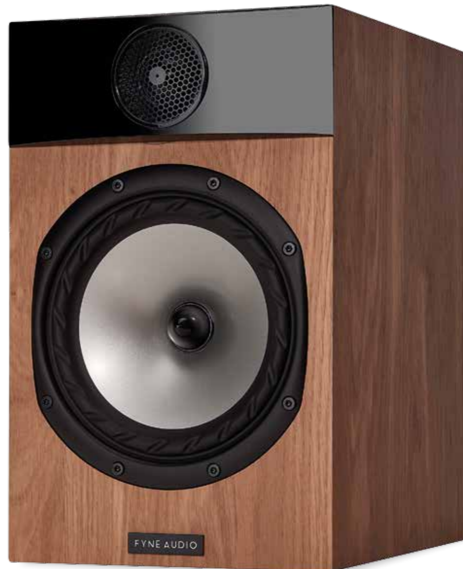
LEFT: The F301's cross-braced MDF cabinet is further reinforced by anchoring up against the rear of the mid/bass unit's magnet. This 150mm unit employs a fibre cone, the tweeter a 25mm polyester dome. Crossover is at 3.2kHz
